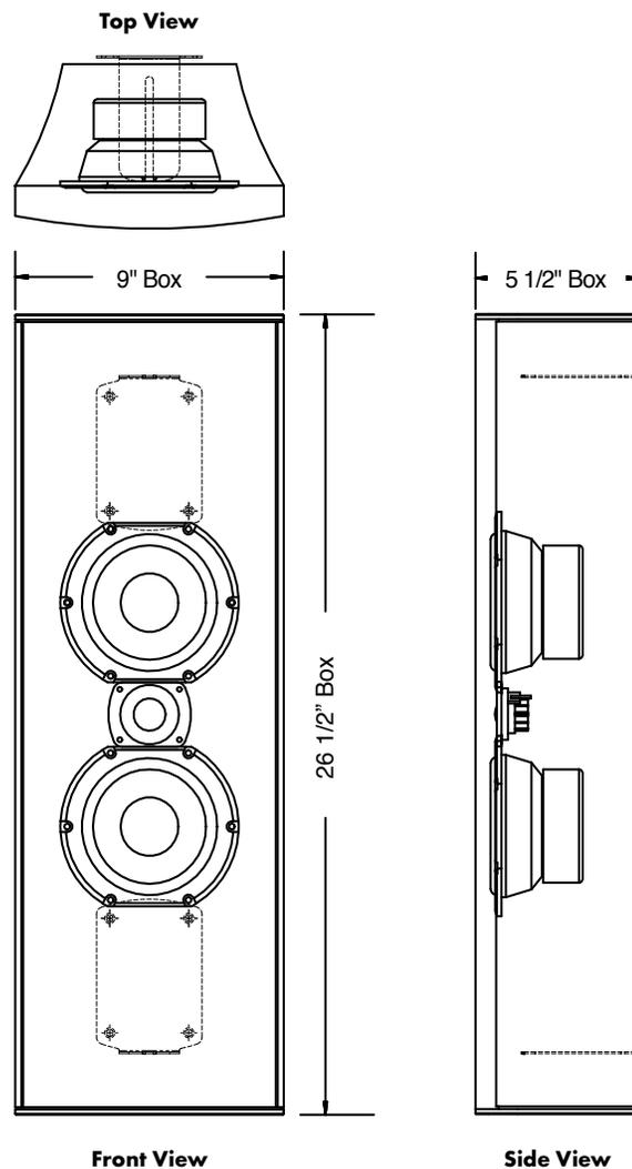
Bracing omitted for drawing clarity
