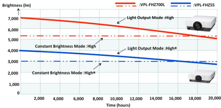
Sony's Z-Phosphor projectors can go 20,000 hours with virtually no maintenance (conditions apply).
