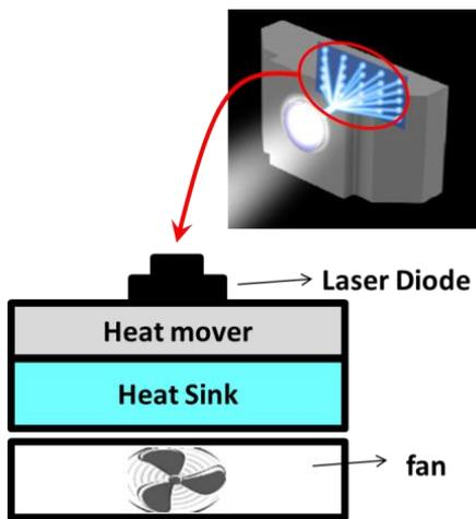
The cooling systems of Sony's laser projectors accommodates all installation angles.\*
