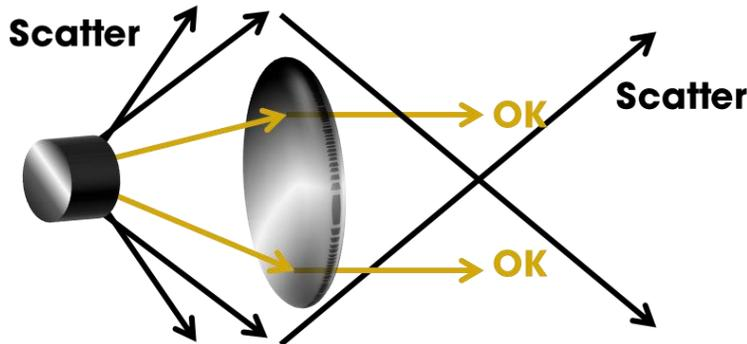
Compared to lasers, LED light sources tend to be relatively large, which incurs light-wasting scatter.
