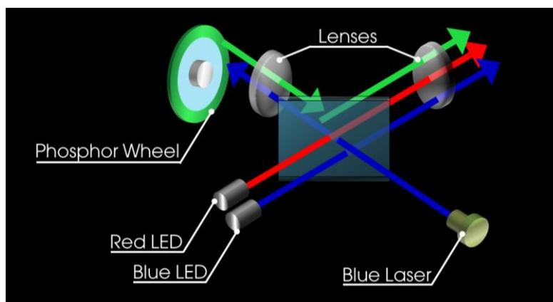
While LED/laser hybrid systems vary, this example is representative. Here the laser is responsible only for Green illumination. Red and Blue are handled by LEDs.
