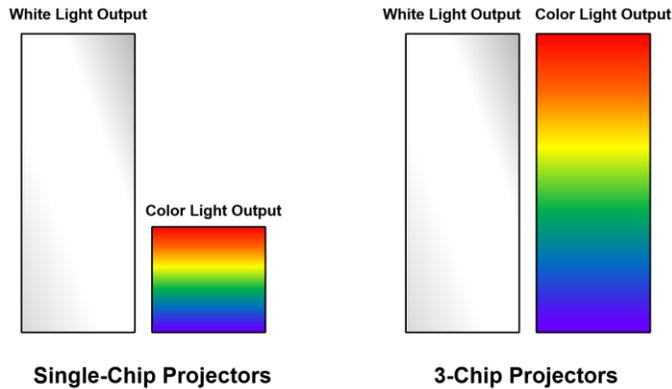
Single-chip projection color light output is just a fraction of the white light output claimed in brochures and ads. For the 3-chip system of Sony laser projectors, the two measures are identical.
