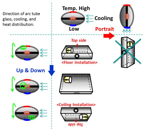
Many lamp-equipped projectors can be tilted vertically (i.e. for floor projection) but cannot be rotated into portrait mode due to limitations in the way lamps can be oriented. Lamps are subject to overheating and failing prematurely when the projector is not installed properly.
