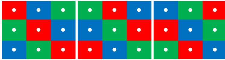
White light output measures nine test points on an all-white screen (left). It's a holdover from the days when computer screens were mostly text on a white background. Color light output measures 27 test points on a sequence of three color screens (right). It's far more representative of today's projector usage.
