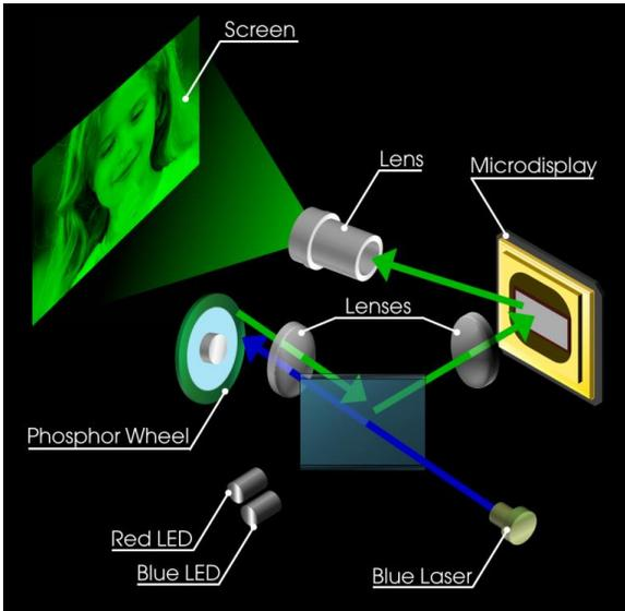
Using a single microdisplay, this LED/laser hybrid system can only present one color at a time—either Red or Green or Blue. In the example shown here, when the laser is active, the projector presents a Green picture.
