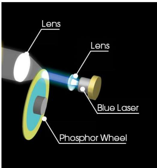
Sony's Z-Phosphor laser light source uses a laser and phosphor wheel to generate the full spectrum of white light. No LEDs are needed.
