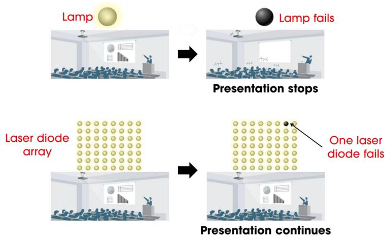
You can present with greater confidence because Sony uses an array of minuscule lasers.
