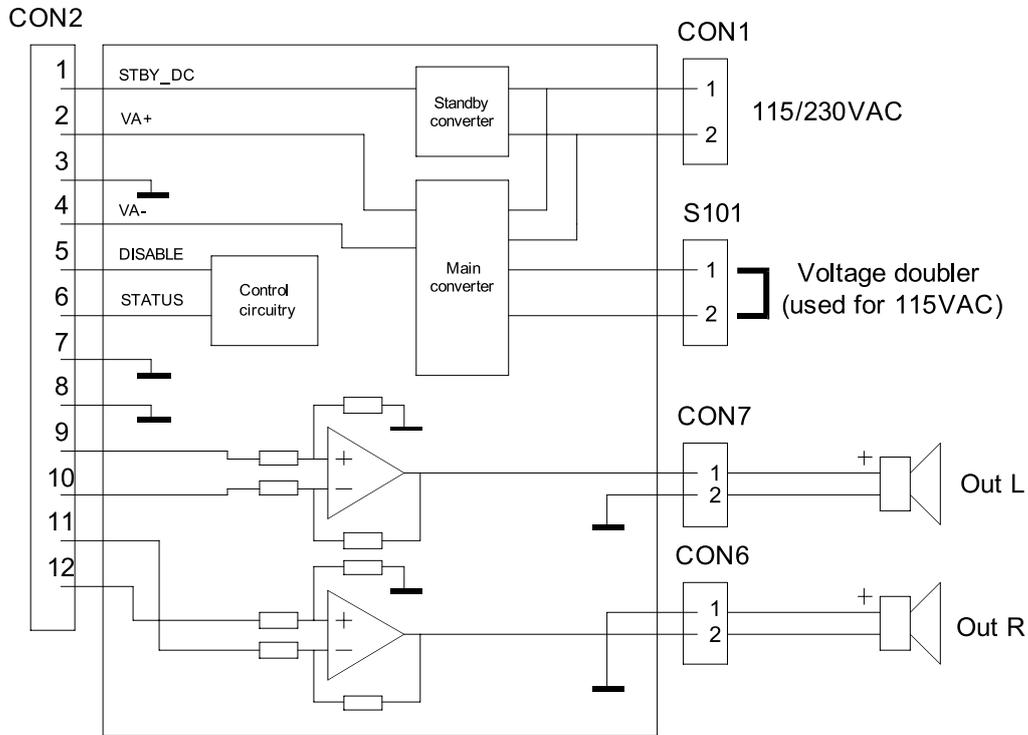
Block diagram amplifier with front end
